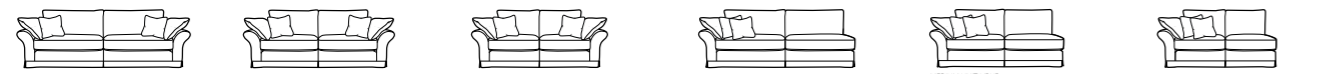
LARGE SOFA H W D SH SW SD AH 87 235 105 48 160 56 59 MEDIUM SOFA H W D SH SW SD AH 87 207 105 48 135 56 59 SMALL SOFA H W D SH SW SD AH 87 175 105 48 100 56 59 LARGE UNIT L/RHF H W D SH SW SD AH 87 208 105 48 170 56 59 MEDIUM UNIT L/RHF H W D SH SW SD AH 87 180 105 48 145 56 59 SMALL UNIT L/RHF H W D SH SW SD AH 87 148 105 48 110 56 59
